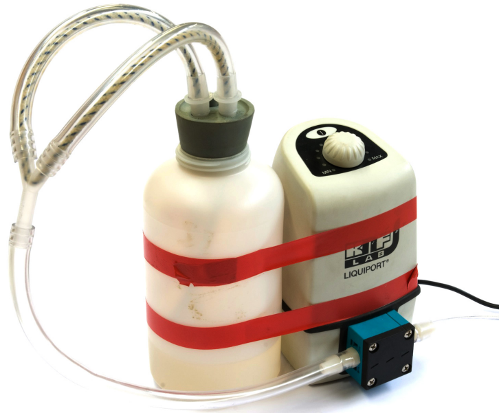
Figure 6.4 – Odour pump and ethanol reservoir.
