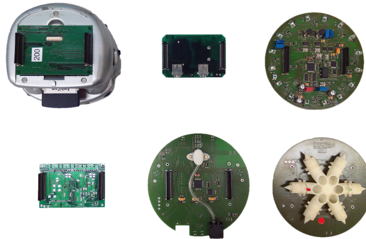
Figure 5.3 – Individual components of our Khepera III stack. Top row: Khepera III robot, power conversion board, relative positioning board. Bottom row: mechanical spacer, odour sensing board and wind sensing board.
